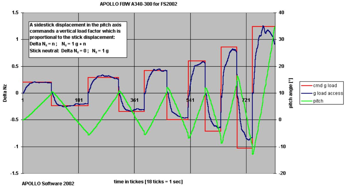
The following typical flight maneuvers illustrate the function of APOLLO's FBW Airbus for FS2002.
